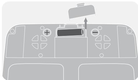
1. Remove the battery door located on the bottom of the feeder. Insert the (+) positive end of the AA alkaline battery (not included) first, then the (-) negative end into the compartment until it clicks into place. Replace battery door. Your feeder is now on!
