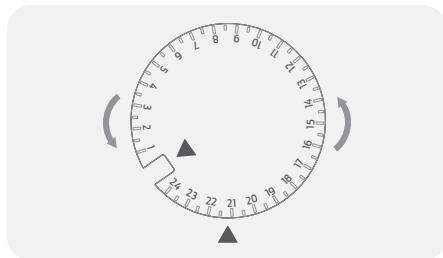
4. Decide on feeding times for your pet and then count how many hours the feeding times are from your CURRENT time – the number of hours is what you will set the timers for. For example, if it's 8 AM and you set one dial to 4 and one to 9, then the corresponding lids will open at 12 pm and 5 pm.
